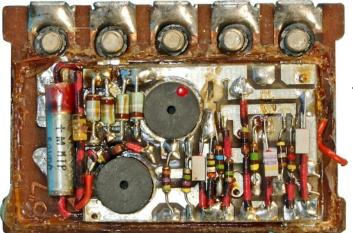
TF-B tx (2B) transmitter 33010 Variation B board glued under a pertinax terminal board prior to being to concealed inside a 5-pt terminal box. (See Chapter 169).
